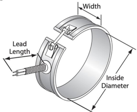
**Fiberglass Leads with Metal Braid-** Specify location and length of leads at time of order.
