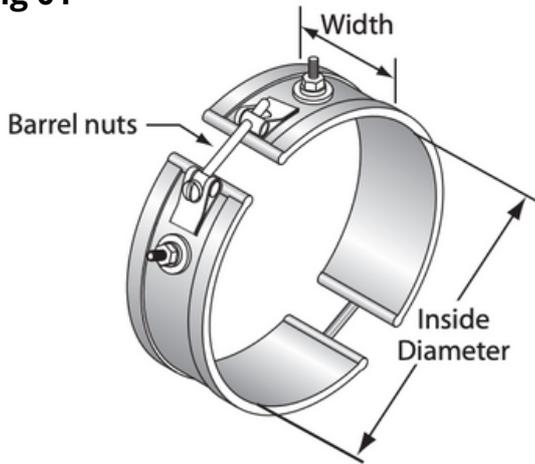
**2 Piece Construction-** Ease of installation in difficult locations. Recommended for diameters larger than 15". Available with any termination or clamping styles.
