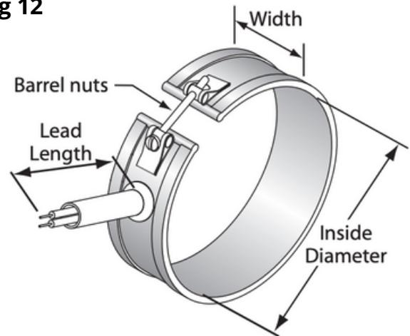
**Fiberglass Leads with Protective Sleeve-** Specify location and length of leads at time of order.
