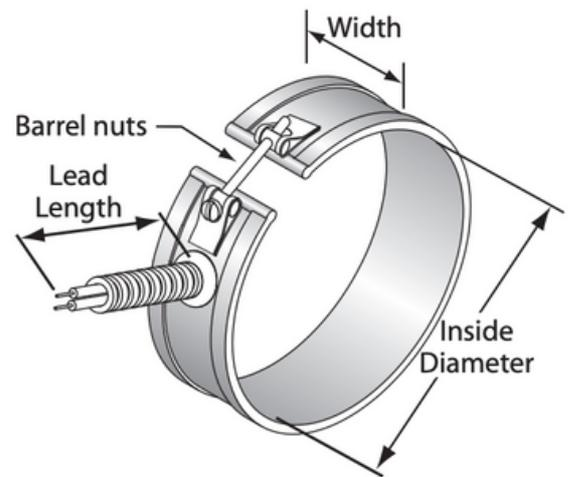
**Fiberglass Leads with Armor Cable-** Specify location and length of leads at time of order.
