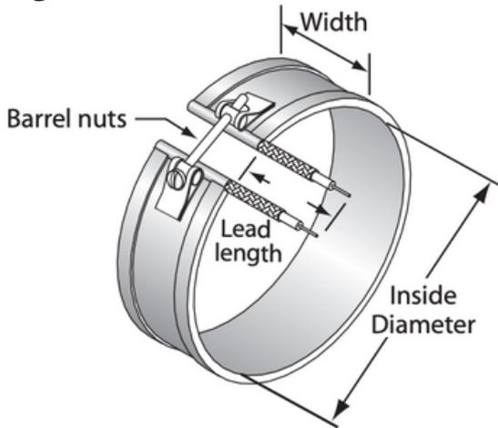
**Nozzle Style-** Fiberglass leads with metal overbraid 12" long is standard
