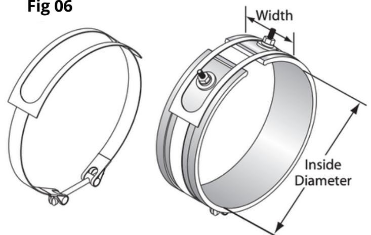
**Separate Strap-** Available in all sizes and configurations. Built-in straps are recommended wherever possible. Typically used in smaller diameters.
