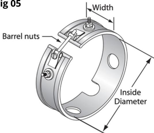
**Holes and Cutouts-** Allow for installation of thermocouples and transducers and give clearance for mounting bolts.
