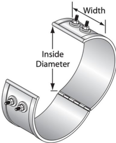
**Expandable or Hinged-** One piece construction used where heater cannot be slid over the barrel or die. Two sets of terminals required. All terminations available
