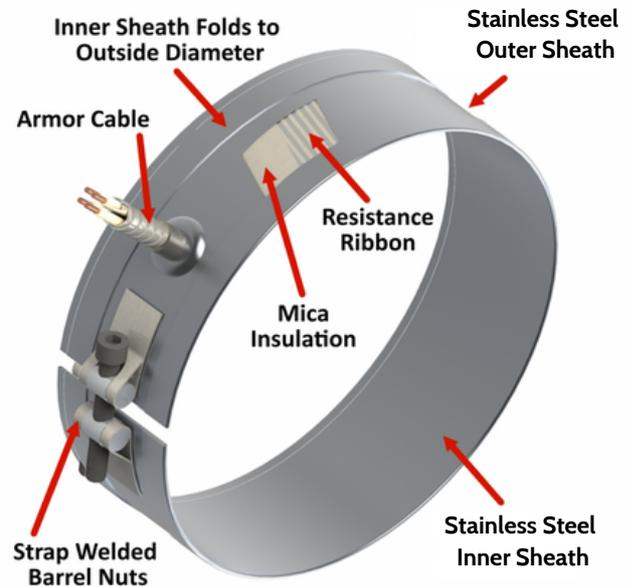
Fig 1. Mica Band Heater Construction
