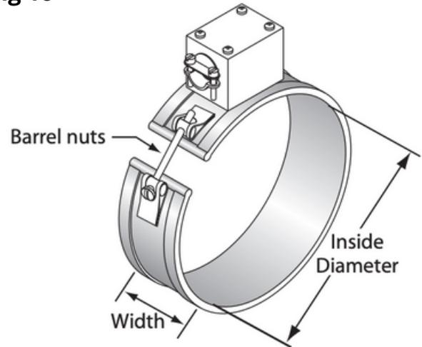
**Sheet Metal Terminal Box-** Available with T2 and T3 threaded terminals.
